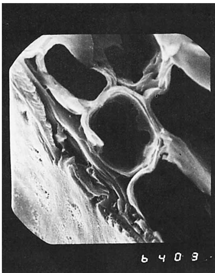
Fig. 1b. Ray-cells of Eucalyptus chips pretreated with HClO-NaClO.
